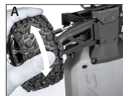
Rotate the rear wheels slowly until the output shaft keys into place.
